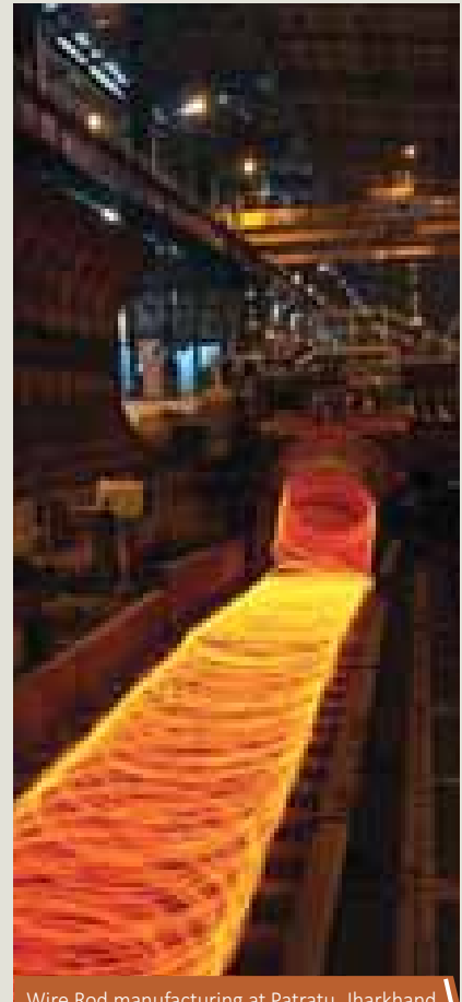
Wire Rod manufacturing at Patratu, Jharkhand
